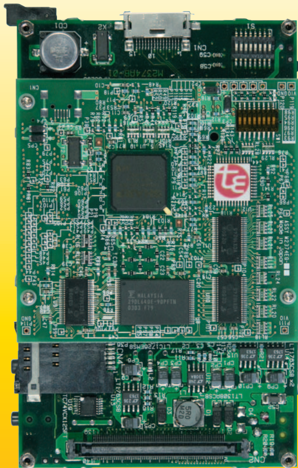
The CPU Board of the T-Engine/ARM922-LH7 Development kit (in full-scale)
