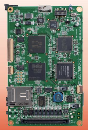
The CPU Board of the T-Engine/SH7760 Development kit (in full-scale)
