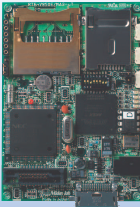
The CPU Board of the \mu T-Engine/V850E-MA3 Development kit (in full-scale)
