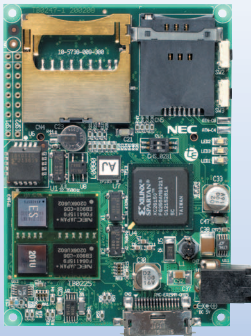
The CPU Board of the \mu T-Engine/VR4131 Development kit (in full-scale)
